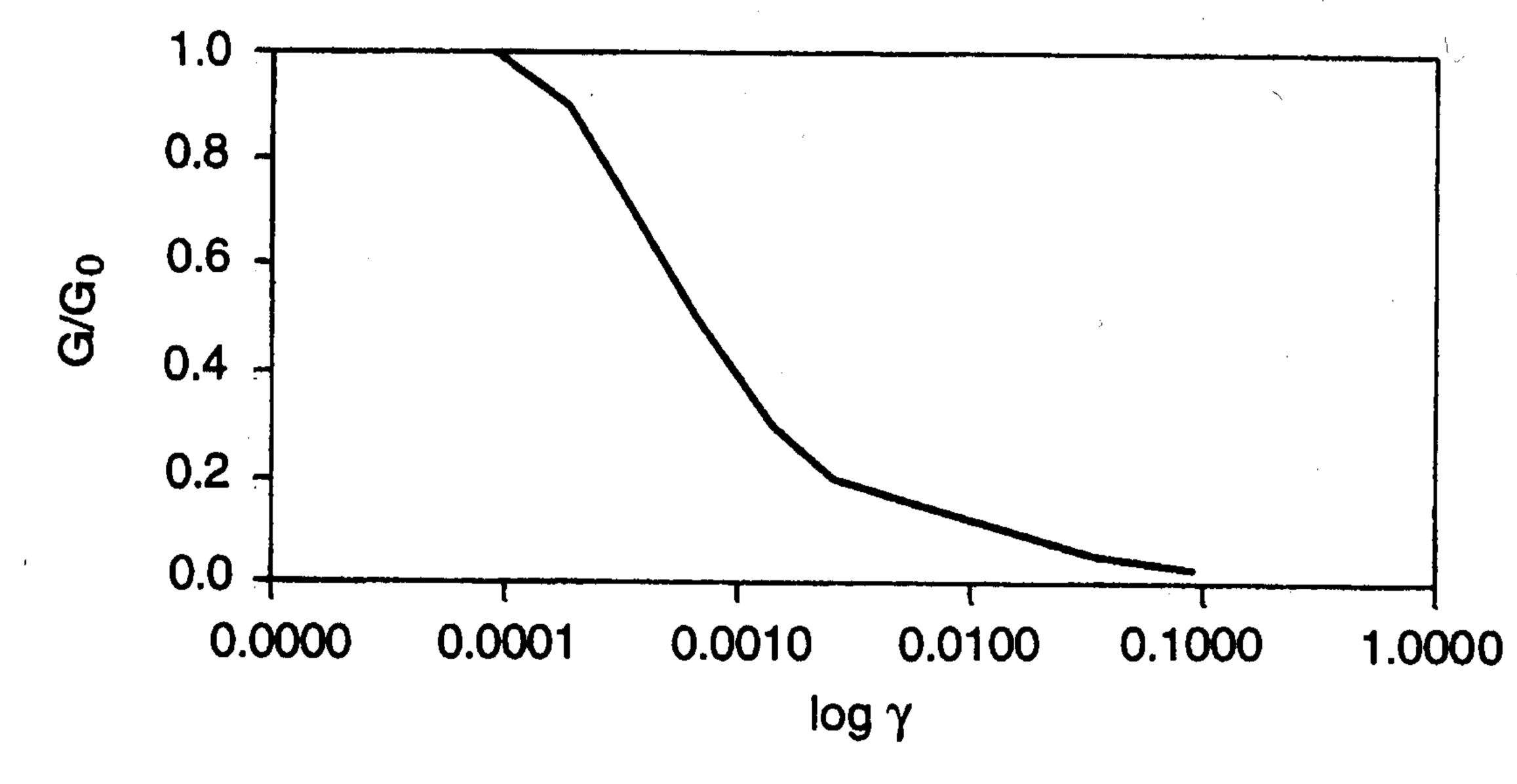
10-surface model used in this study. (In Fig 1,  $G_0$  is the shear modulus at very small strain and  $\gamma$  is the shear strain.)
