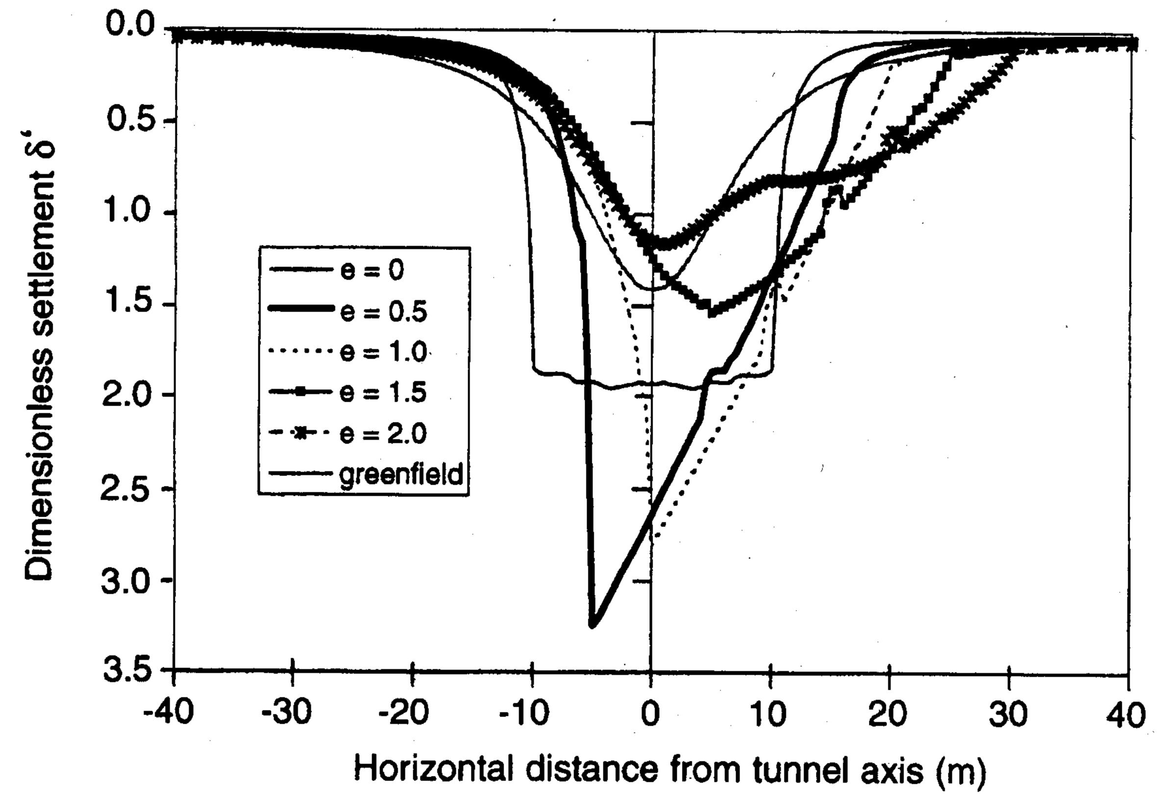
Fig 15. Settlement profiles for varying facade position (light facade,  $\gamma_b t =$  $10.0kN/m^2$ )
