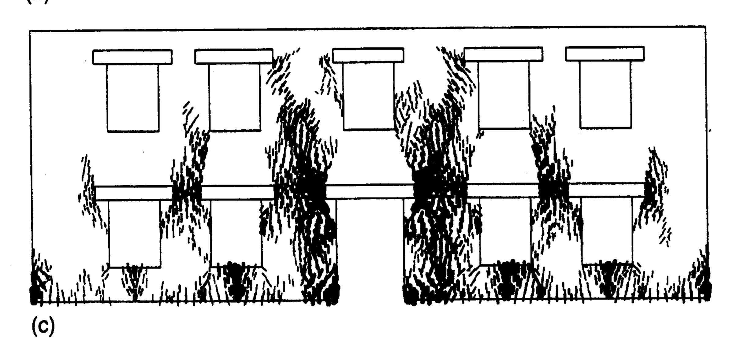
This process is illustrated in Fig 18. Clearly, stress arches cannot be formed when e=2, in the tensile horizontal movement area of the settlement trough, as there is no line of thrust available within the facade to the ground.
