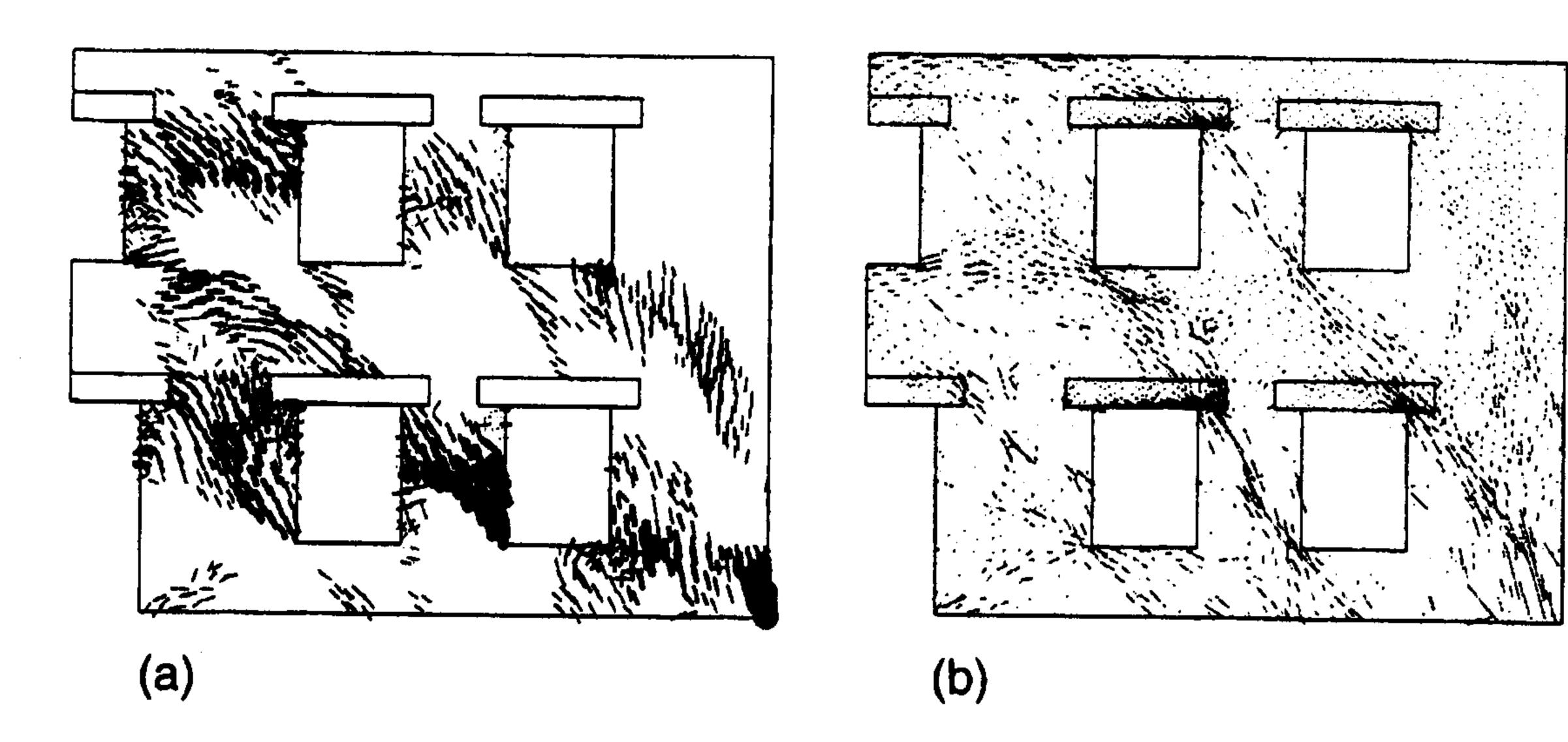
are shown in Fig 7(a) and (b). Again, the stress trajectory plots show that the differential settlements force an arching effect in the masonry material of the facade. Two 'stress arches' are visible in the uncoupled analysis, while three are visible in the coupled analysis.
