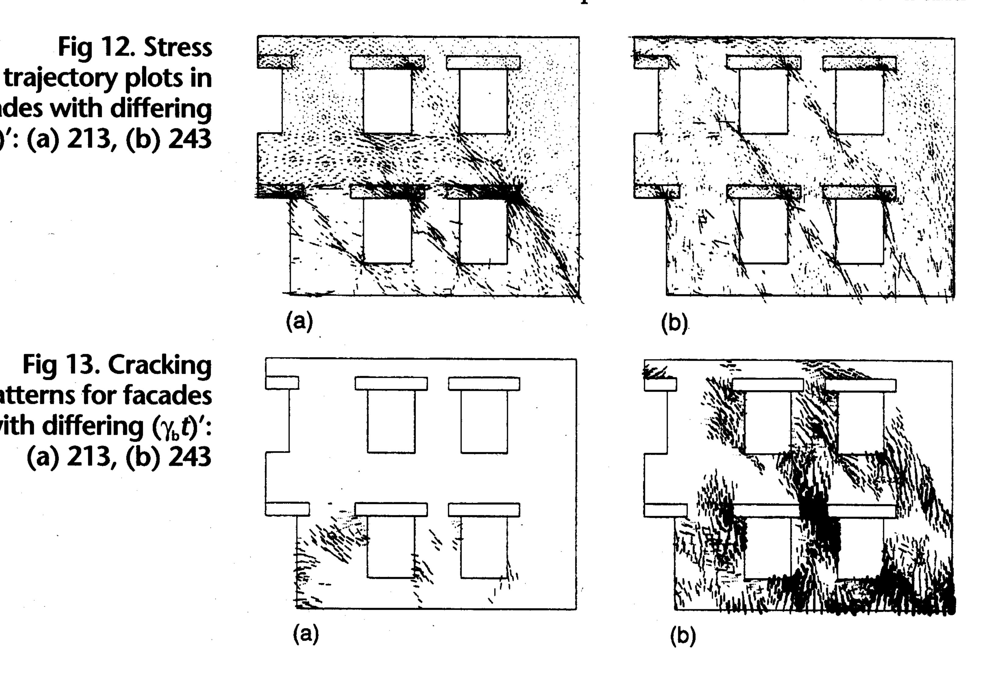
Fig 13. Cracking patterns for facades with differing  $(\gamma_b t)'$ : (a) 213, (b) 243
